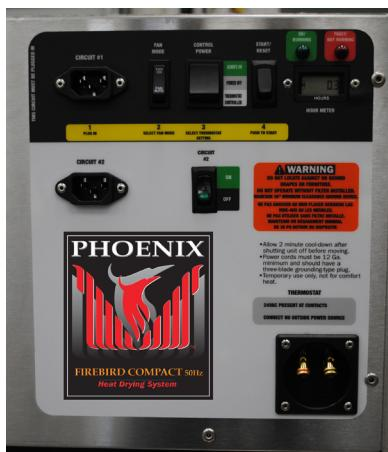
**Start/Reset Switch:** The START/RESET Switch is used to enable the Compact to produce heat. If at any time power to the control circuit is lost or if a fault condition occurs, the Compact will go into the FAULT/NOT RUNNING mode. Pushing the START/RESET switch will energize the control circuit and restart the Compact.
